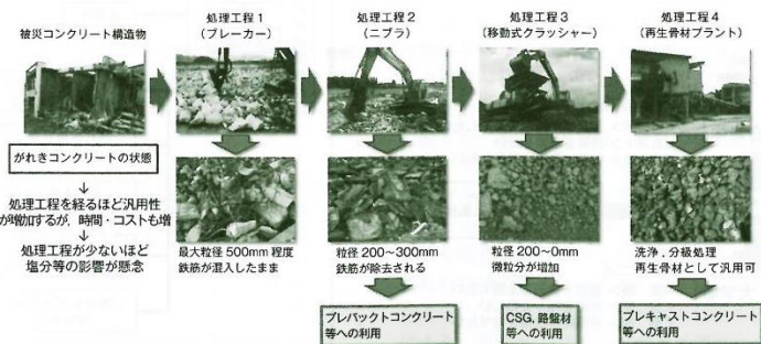
Fig. 5 Quality and process of concrete rubble
